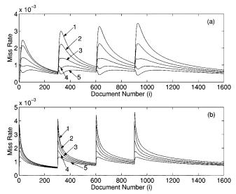
Fig. 4. Cache miss rates for individual documents—inhomogeneous case. (a)  $z_k = 1$ . (b)  $z_k = 0.6$ . Curve 1: cache miss rate at leaf level cache. Curves 2, 3, 4, and 5: cache miss rates at the root cache for  $C_0 = 800$ , 1200, 1600, 2000.
