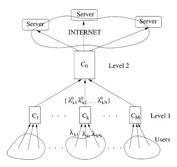
Fig. 1. Two-level hierarchical web caching structure.
