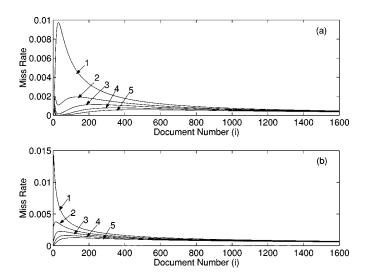
Fig. 3. Cache miss rates for individual documents—homogeneous case. (a)  $z_k=1$ . (b)  $z_k=0.6$ . Curve 1: cache miss rate at leaf level cache. Curves 2, 3, 4, and 5: cache miss rates at the root cache for  $C_0=800$ , 1200, 1600, 2000.
