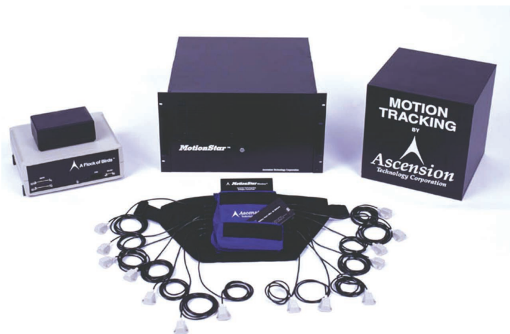
Figure 2. MotionStar DC magnetic tracker, a precision system used in motion capture for computer animation, tracks the position and orientation of up to 108 sensor points on an object or scene. Key components include (left and right) the magnetic pulse transmitting antennas and (center) the receiving antennas and controller. Image courtesy of Ascension Technology Corporation.
