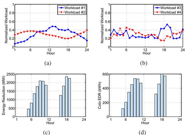
Fig. 1. Workload and energy reduction target. (a) & (b) Normalized workload trace, (c) Energy reduction target at PJM, (d) Scaled energy reduction target for colocation.
