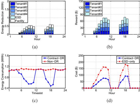
Fig. 4. Comparison. (a) Energy, (b) Total reward, (c) Energy consumption, (d) Colocation's cost for demand response.
