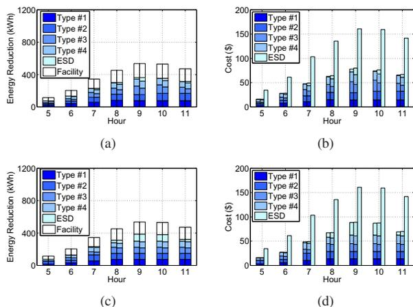
Fig. 2. Energy reduction and cost for Discrete-Complete and Discrete-Incomplete types. (a) & (b) 10 tenants, (c) & (d) 30 tenants.
