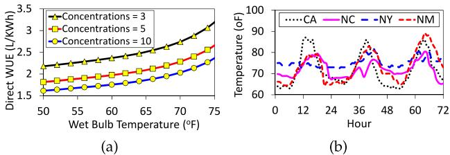
Fig. 1. (a) Direct WUE versus outside wet bulb temperature [44]. Lines/markers represent modeled/measured values. (b) Three-day outside temperature starting from July 1, 2012 [11].
