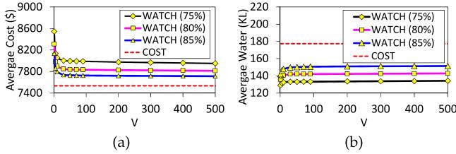
Fig. 6. Cost-water tradeoff under different water caps. (a) Operational cost. (b) Water consumption.
