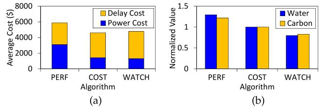
Fig. 12. Comparison among PERF, COST, and WATCH. (a) Operational cost. (b) Water consumption and carbon emission.
