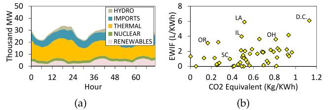
Fig. 2. (a) Three-day fuel mix data of California ISO starting from Sep 1, 2013 [1]. (b) State-level EWIF versus CO<sub>2</sub> emissions in the US [45], [47].
