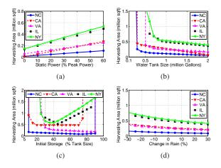
Figure 4: Impact of (a) power proportionality, (b) water tank size, (c) initial water storage, and (d) annual rainfall.
