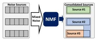
Fig. 8. Illustration: NMF converts the 15 noise sources into 3 consolidated sources.
