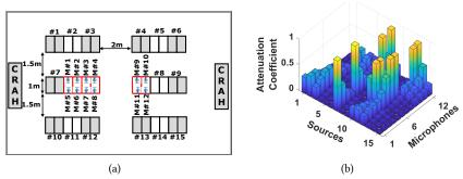
Fig. 29. Simulation settings for robustness study. (a) Simulated data center layout. (b) Attenuation modeled using the inverse square law.
