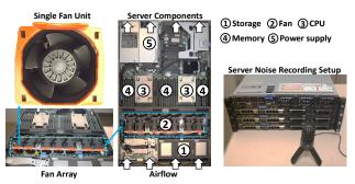
Fig. 4. Inside of a Dell PowerEdge server and a cooling fan. The server's cooling fan is a major noise source.
