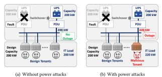
Figure 1: Loss of redundancy protection due to power attacks in a Tier-IV data center.
