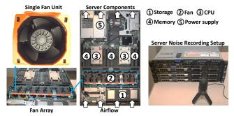
Figure 4: Photo of inside of a Dell PowerEdge server and a cooling fan. The server's cooling fan noise is a major source of noises.
