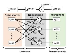
Figure 21: Noise energy mixing process.
