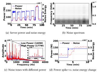
Figure 18: Experimental results on SuperMicro servers.
