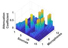
(b) Attenuation modeled using the inverse square law Figure 29: Simulation settings for robustness study.
