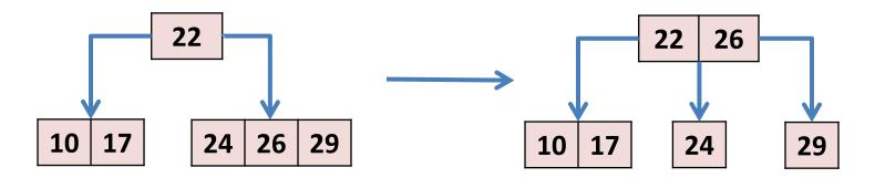
• If we find a 3-node being parent to a 4-node, we transform the pair into a 4node connected to two 2-nodes, by pushing up the middle key of the 4-node.
