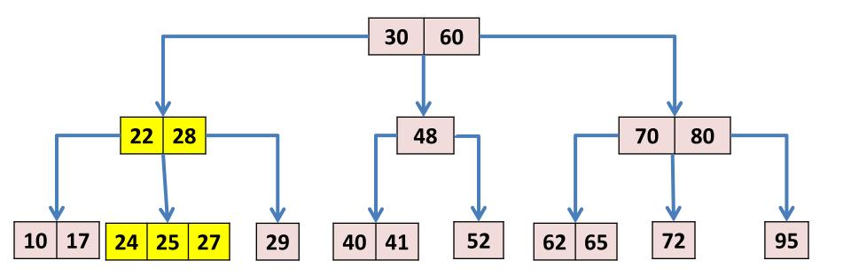
• Found a 3-node being parent to a 4-node, we must transform the pair into a 4-node connected to two 2-nodes.
