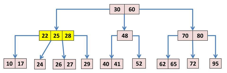
• Found a 3-node being parent to a 4-node, we must transform the pair into a 4-node connected to two 2-nodes.
