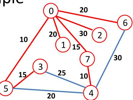
1. Start by adding vertex 0 to the MST (minimum-cost spanning tree).
