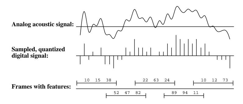
Frame features are typically formants—peaks in the power spectrum
