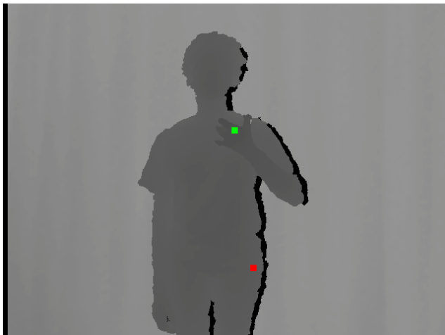
Figure 7: Failure of the skeleton tracker after the signer’s arms were at her side. The red square is the tracker hand position estimate. The green square is the centroid of the hand bounding box.
