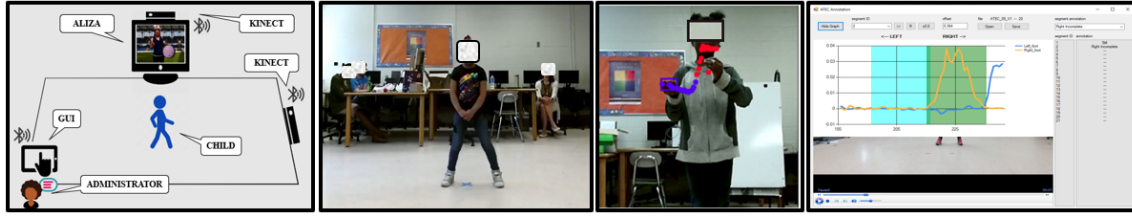
Figure 3: The ATEC setup includes two Kinect cameras, a large screen and a tablet interface for the administrator. Administration takes place in classroom environments. Annotation software was developed to enhance manual scoring and annotate the collected data, given the task rules and the cognitive measures to be assessed.
