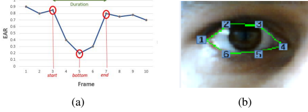
Figure 3. (a) The EAR sequence during an entire blink and the start, bottom and end points. (b) The eye landmarks to define EAR for each frame.
