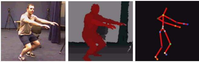
Fig. 3. Example of full body tracking provided by Kinect SDK. The left image shows the RGB color frame of a subject performing a RA exercise. The middle image shows the depth sensing information of the same frame where the pixels corresponding to the tracked subject have been marked in red. The right image shows the skeletal information extracted by Microsoft Kinect SDK.
