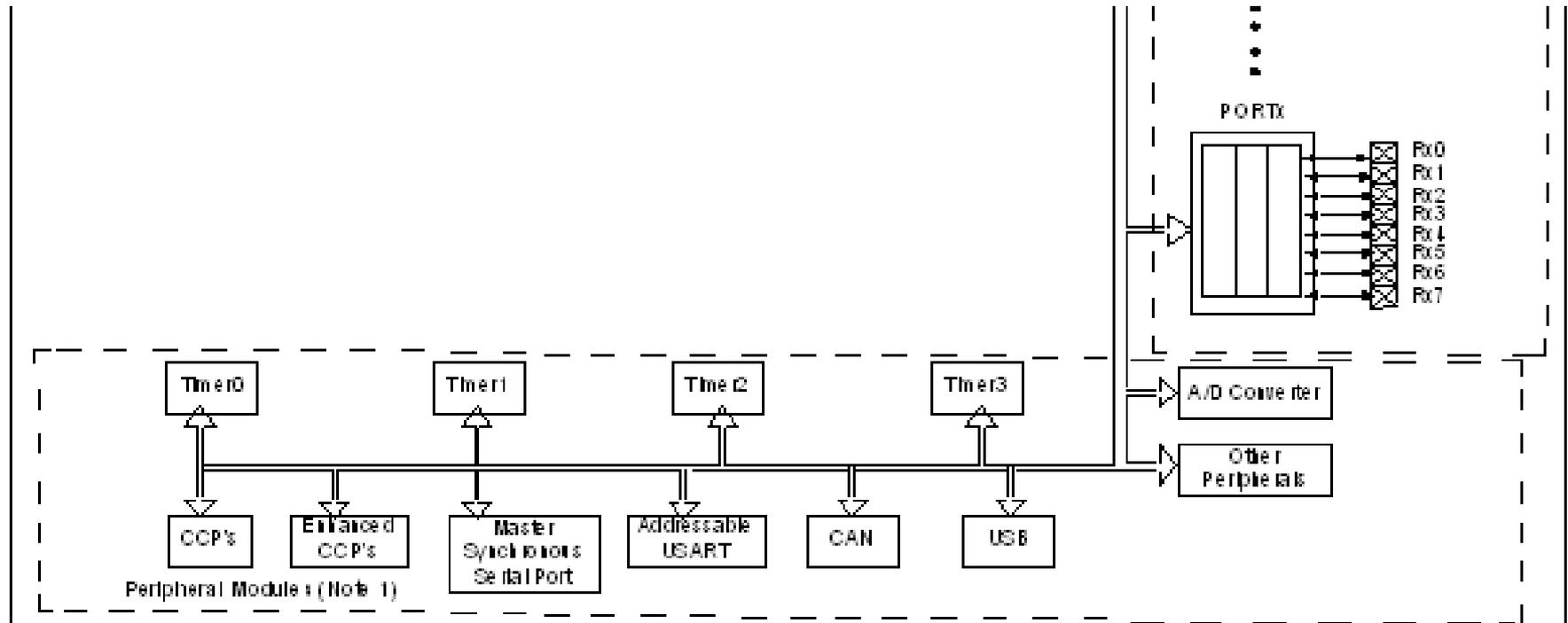
**Note 1:** Many of the general purpose I/O pins are multiplexed with one or more peripheral module functions. The multiplexing combinations are device dependent.
