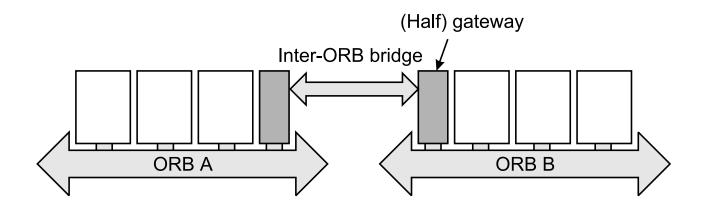
**Solution:** Object references passed from one ORB to another are transformed by the bridge through which they pass (different transformation schemes can be implemented)
