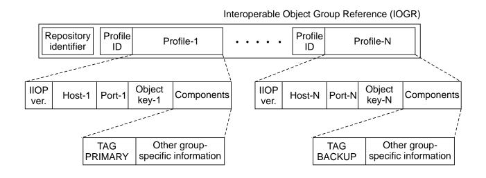
**Note:** IOGRs have the same structure as IORs; the main difference is that they are *used* differently. In IORs an additional profile is used as an alternative; in IOGR, it denotes another replica.
