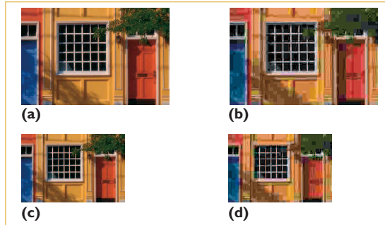
Figure 4. MobiGATE's adaptation effects on image data. (a) The original image (12.9 Kbytes) passes through (b) the image down sampling streamlet (3.18 Kbytes) and (c) the image lower size streamlet (8.63 Kbytes), resulting in (d) a smaller, lower-quality image (2 Kbytes), which the client receives on a smaller display.
