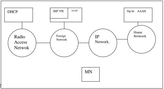
MN is the mobile node that allows users to communicate and also provides means of interactions and control between users and the network.
