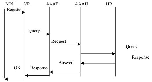
First the MN sends a SIP REGISTER Message to the VR with its new IP address; this is done through the SIP proxy Server Address obtained from the DHCP messages. The VR queries the AAA entity (Authorization, Authentication, Accountability) .The AAAF entity of the visited network queries the AAA entity (AAAH) of the home network to verify MNS credential sand rights. The AAH queries the HR and depending on the response from the HR it sends a response to the AAAF.
