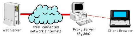
The fig depicts the architecture of Pythia. Rather than fetching a URL directly from the appropriate server, the fetch request is passed on to the proxy. The proxy obtains the document from the server on the client's behalf, and forwards it to the client. Pythia can run anywhere inside the wired Internet.
