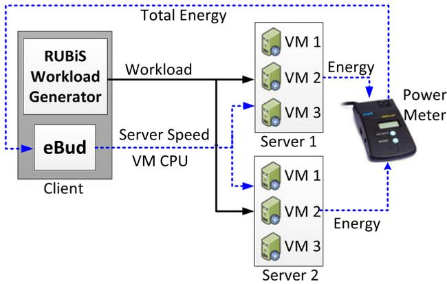
Fig. 8. Experiment setup for validating eBud.
