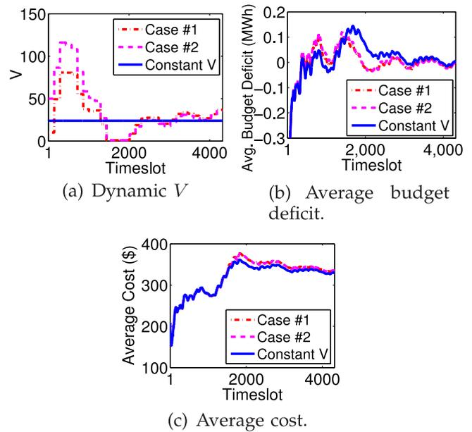
Fig. 4. Dynamically updating  $V$  every day. Case #1: initial  $V = 10$ . Case #2: initial  $V = 50$ . Constant  $V = 24$ .  $\alpha = 50$ .
