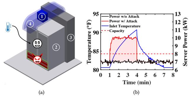
**Figure 1: (a) Layout of a multi-tenant edge data center. ① Air conditioner. ② Server racks. ③ Return air duct. ④ Supply air duct. (b) Power and inlet temperature trace during an attack.**
