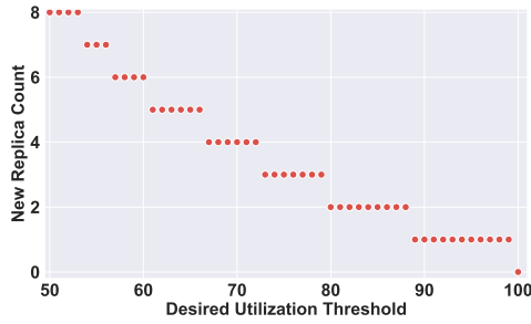
Fig. 3: HPA calculates new instances based on desired utilization value and current utilization
